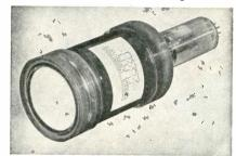
tions. A coaxial electron gun system eliminates trapezoidal distortion of the scanning pattern. Special features: Full daylight viewing by image intensification and the ability to write, store and erase information at will. A display exceeding 4000 ft .lamberts brightness is obtained at a phosphor voltage of 8.5 kv. The tube fits within standard case dimensions for a 2% in. dial instrument and meets MIL-E-5400. ITT Laboratories, 3700 East Pontiac St., Fort Wayne, Ind.
