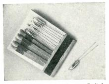
light weight or space factor. Switching action is SPST; differential angle is 15°. AC load at 115 v. and 230 v. is 0.1 a; dc load at 115 v. and 230 v. is 0.1 a; lamp load is 10 w; Locked rotor rating: ac inrush at 115 v. is 1 a, at 230 v. is 0.5 a; dc inrush at 115 v. is 1 a, at 230 v. is 0.5 a. 8 in. length of #26 PVC is the standard lead wire. Gordos Corp., 250 Glenwood Ave., Bloomfield, N. J.
