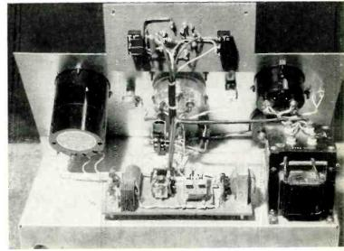
Fig. 4: Regulated plate power supply is mounted under the chassis shown in Fig. 3. Shaft adjusts voltage from front panel
