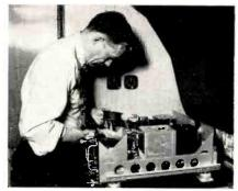
Project Engineer, William Plice, installs magnetic tape in Flight Recorder which monitors 65 flight condition variables. Analysis of performance provides statistical means to determine when maintenance is needed. Minneapolis-Honeywell, Regulator Co., developers, demonstrated the recorder for Federal Aviation Agency Officials.
