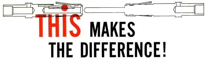
Right here in the socket contact lies the heart of the **AMPin-cert Connector** line: the AMP cantilever spring. Seated in the slot of the socket to meet the pin shaft, it is your key to top connector reliability.
