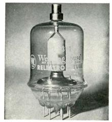
of 75 w are applicable for continuous commercial service. A max. signal power dissipation of 125 w applies for SSB service. Performance extends to 175 MC. Reliable service and high efficiency are obtained by the thoriated tungsten cathode. Also, good isolation between input and output circuit is provided by tube's construction. A rugged screen grid gives ample dissipation for all types of communication service. Westinghouse Electric Corp., Electronic Tube Div., P. O. Box 284, Elmira, N. Y.
