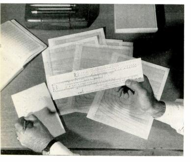
New slide rule eliminates need for graphs and tables in filter calculations. Combination of special and conventional scales permit answers to all filter calculations to be read directly from the rule.
