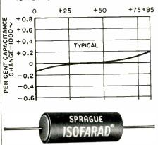
A new duplex plastic film dielectric developed and patented by the Sprague Electric Co. displays practically a zero temperature coefficient of capacitance over operating ranges up to +85 C. The retrace on return to room temperature is within + 0.10 %.
