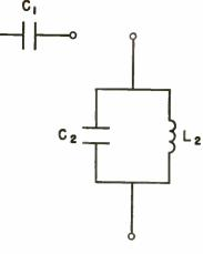
The accuracy test calculations were made for this type of three-element section.
