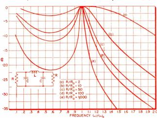
Fig. 3: Use of a matching network to provide appropriate selectivity for a three-element network with equal terminations.
