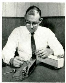
General Electric Development Engineer, Earl Bond, plans typical layout for a small radio using new compactrons. Two of the devices replace five con-miniature electronic tubes. Case under his left hand shows how a compactron radio may look—virtually all speaker.
