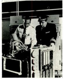
SINS-(S) hips (1) nertial (N) avigation (S) ystems will guide Polaris subs and pinpoint their positions for missile launchings. Its three units sense movement and translate it into heading, speed, and position. Developed by Sperry Gyroscope Co., Marine Div., Syosset, N. Y., the system must operate for long periods of time compared to missile systems.
