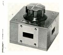
excellent isolation and high power capacity. Series 641 waveguide switches cover the frequency ranges from 3.95 to 40 KMC and each switch operates over the full waveguide bandwidth. Max. vswr is 1.10. The min. isolation is 60 db for frequencies from 3.95 to 26.50 KMC and 50 db from 26.50 to 40 KMC. FXR, Inc., 26-12 Borough Place, Woodside 77, N. Y.
