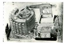
sequence control, totalizing, sampling or single point selection. It transfers from Position 10 to Position 1 without special circuitry. C. P. Clare & Co., 3101 Pratt Blvd., Chicago 45, Ill. Circle 177 on Inquiry Card
