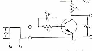
Fig. 15: This saturated switching circuit has a "speed-up" capacitor across the large resistor in series with the base. The capacitor tends to reduce the total switching time considerably.
