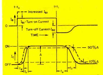
Fig. 10 (above): Effects of increased turn-on current with turn-off current present. The latter is a transient, present only while the transistor is in storage. It is not a steady-state value of current.
