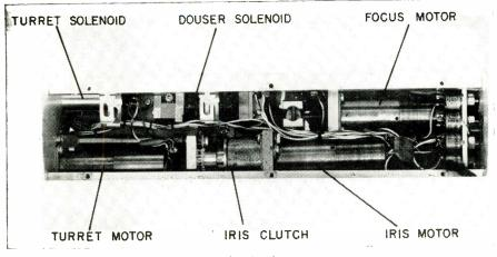
Fig. 9: Remote control functions are handled by these accessory motors.
