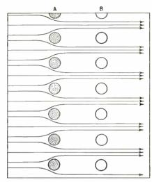
The "blocking back" concept is used by General Electric's new 6FG5. An "extra" shadow grid (A) diverts electron flow around screen grid (B) thus drastically reducing screen current. With this design, the screen grid can be tied directly to the plate voltage, eliminating dropping resistors and by-pass capacitors. Reduction of screen current also permits exceptionally low-noise pentode operation.
