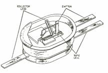
0.180 x 0.060 in. About 42 enclosures can be mounted on 1 sq. in. multi-element wafer, and still add only about 1/16 in. to its thickness. Featured is a cold welded, metal-toglass, hermetically sealed package providing a min. seal length of 0.050 in. It will house any type of standard computer transistor. Philco Corp., Lansdale Div., Lansdale, Pa. Circle 178 on Inquiry Card
