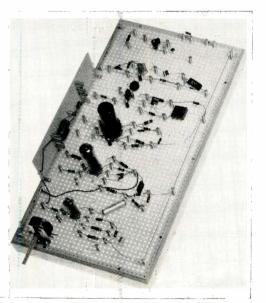
such a way that wire leads are held rigidly in place without soldering. Contact resistance is less than 0.002 ohms.
