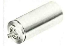
torque at stall, 1.3 gm. cm.<sup>2</sup> rotor moment of inertia, 3.5 w per phase stall power, 120 + J1780 = 2175ohms impedance at stall, 115 v. fixed phase and 115/57.5 v. control phase voltage and 0.053 a per phase current at stall. 115 v, 400 CPS generator has 3.05 w input, 0.5 v per RPM min. at 25°C output voltage, 10° max. phase shift, and 1200 ohms output impedance. John Oster Manufacturing Co., Avionic Division, 1 Main St., Racine, Wisc.
