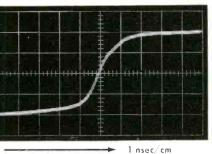
Typicol waveform of gallium arsenide tunnel diode in T≅ktronix Tunnel Diode Risetime Tester (port number © 3-029), Price \$50.
