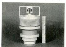
and long life. In plate-and-screen pulsed service, the new tetrode is rated for 50 kw of peak power at 500 MC, with a power gain of 20 and a pulse width of 15  $\mu$ sec. It is capable of providing useful output up to approx. 1500 MC. It may also be used as a grid-pulsed r-f amplifier or as a grid-and-screen pulsed r-f amplifier. General Electric Co., Schenectady 5, N. Y.
