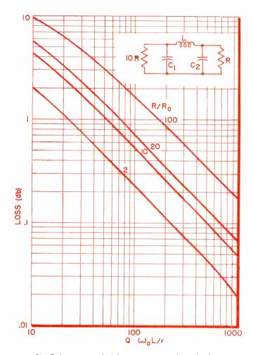
Fig. 7: Loss at matched frequency-unequal terminations.
