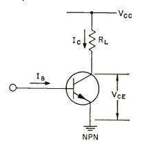
Fig. 8 (left): This circuit may be used for determining switching times between the ON and OFF points of a saturated switch.
