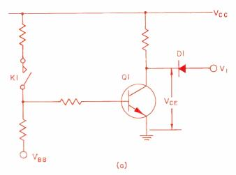
Fig. 17: Examples of non-saturated switches with current drive.
