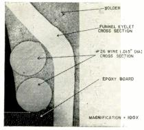
Fig. 7: Photomicrograph of solder joint achieved by process of wave soldering.
