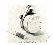
cial 60-cycle ac Timing Motor, currently being used in many applica-tions, is only % in. long. Available in voltages ranging from 6 to 230 v. at 20 ma max., the unit's rotor speed is 300 rpm with output speeds of 300 rpm to 1/6 rph. Max. temp. rise is only 40°C. Power input is 2.5 w max. A. W. Haydon Co., 232 N. Elm St., Waterbury, Conn.
