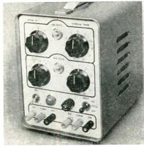
off cycle. Applications are in environmental testing, life cycle test, electromechanical testing, and photography. Control relay has 15 a DPDT contacts with 1500 vac insulation. Max. and min. time rates for either the on or off cycle are approximately 4 min. to 60 #sec. Technitron Co., 7088 Osbun Rd., San Bernardino, Calif. Circle 223 on Inquiry Card
