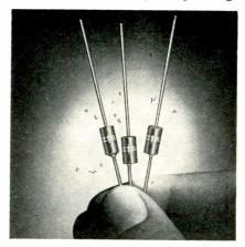
from -65 to +130 °C. Each junction is encapsulated in a stable, high temp. non-metallic case. International Rectifier Corp., 1521 E. Grand Ave., El Segundo, Calif. Circle 181 on Inquiry Card
