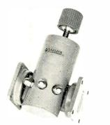
which varies from 29 to 36 MC over the band. The insertion loss at Fo -60 MC is 21 db min. Unit, part number 60017, is manufactured in aluminum and has been designed to withstand severe shock and vibration environments. The insertion length or dimension from flange to flange is 2.75 in. and tuning is accomplished through a precision micrometer type drive screw with a positive locking device. Waveline Inc., Caldwell, N. J. Circle 203 on Inguiry Card
