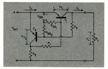
$T_1$  is a germanium type, the forward emitter-base drop is somewhat less than that for a silicon junction  $(D_1)$ . When  $R_4 = 0$  the maximum current passed by  $T_1$  is limited only by the criterion:
