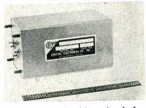
the aircraft and citizen band frequencies. It was designed to carry high power in the order of a 75 w peak and 25 w normal and can be driven from source impedances of between 5 to 10 ohms. Output is to the transmitter's loop antenna. Attenuation is 50 db down at the 3rd Harmonic. Attenuation is held to less than 1 db up to 60 KC and less than 3 db at 65 KC. Control Electronics Co., Inc., 10 Stepar Place, Huntington Station, L. I., N. Y.
