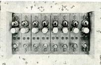
the flore 260 systems requiring a simple one input. one output unity-gain unit; Type VA-P-102 (Sync Adding) plugs into 1 of the positions, when sync-adding is required, allowing the addition of sync to 1 or any number of the remaining 7 VA-P-101 units; Type VA-P-103 (Video Distribution) is a one input, one output unit with nom. gain of +3db; and Type VA-P-201 is a multiple output type for simultaneously feeding 3 identical signals to several different points. The Daven Co., Livingston, N. J.
