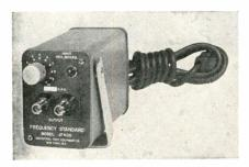
115 v. 60 CPS line. Specs are: frequency, 400 CPS; accuracy,  $\pm 0.1\%$  at 25°C; temp. coefficient, 0.002%/degree °C approx.; output voltage, variable 0-5 v. (no load); recommended load impedance, 0.5 megohm or higher; distortion, 1% approx.; power, 115 v., 60 CPS, 15 w; output, binding posts. Industrial Test Equipment Co., 55 E. 11th St., New York 3, N. Y.
