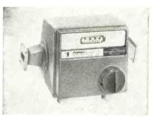
tenuation range of 60 db and a max. vswr of 1.15. Value of attenuation is determined by angular position of a resistive film with respect to the waveguide and is independent of frequency. All 9 units feature small insertion length; 60 db range; tape readout; built-in height adjustment; and low insertion loss. PRD Electronics, Inc., 202 Tillary St., Brooklyn 1, N. Y.
