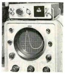
tive oscilloscope may be used for current and voltage wave forms. It creates a sharp representation of the entire critical region of the forward characteristics curve rather than just a portion of that curve. With an external decade box shunted across the horizontal terminals, it is practical to read the actual negative resistance at any point. Texas Instruments Incorporated, Geosciences and Instrumentation Div., Instrumentation Product Group, 3609 Buffalo Speedway, Houston 6, Texas.
