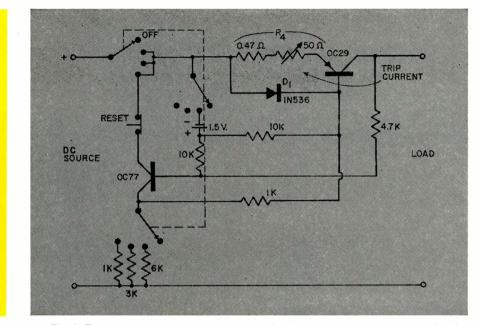
Fig. 4: Triggering device in series with T1 lets bistable circuit be used as a circuitbreaker
