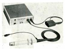
wire, providing a voltage output which is quickly and easily read on a VTVM or oscilloscope. The instrument's 1 mv to 1 ma unity conversion permits direct readings in milliamperes on voltmeters or oscilloscopes. Bandwidth is 20 CPS to 15 MC, permits oscilloscope viewing of complex current waveforms with rise time as fast as 0.08 μsec. Hewlett-Packard Co., 275 Page Mill Rd., Palo Alto, Calif.
