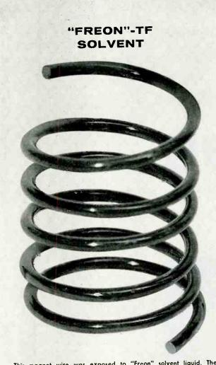
This magnet wire was exposed to "Freon" solvent liquid. The "Glyptal" coating on this wire is completely unaffected by "Freon"-TF. ORDINARY CHLORINATED SOLVENT
