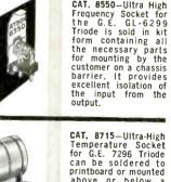
CAT. 8715--Ultra-High Temperature Socket for G.E. 7296 Triode can be soldered to printboard or mounted above or below a chassis. High Alumina insulating material; contacts gold plated Inconel-X. For continu-ous operation at ous operation at 1000° F (538° C),
